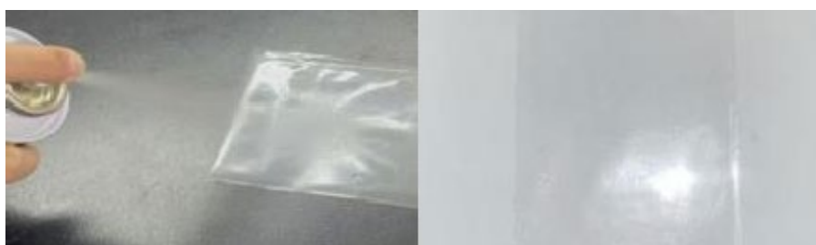
Fig. 7. Evenly sprayed waterproof coating and photos of the finished product.
