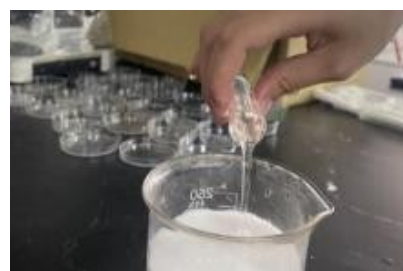
Fig. 4. Mixing operation diagram of adding resin in a gradual pouring manner.
