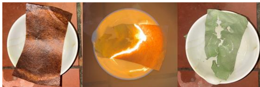
Fig. 5. Left to right: Flash paper infused with \text{CrO}_3 is ignited using a lighter in a porcelain crucible, triggering self-sustained combustion that produces a lightweight \text{Cr}_2\text{O}_3 green pigment within seconds.
