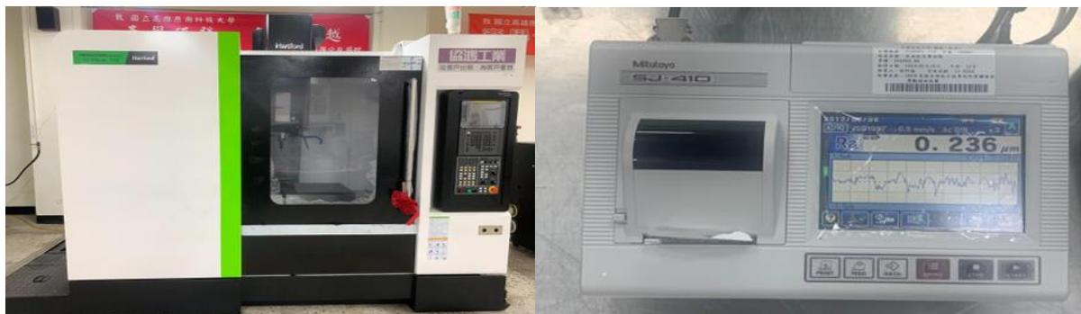
**Fig. 2.** Experimental equipment (a) CNC processing machine S-Plus 10 (b) Surface roughness measuring instrument SJ-410.
