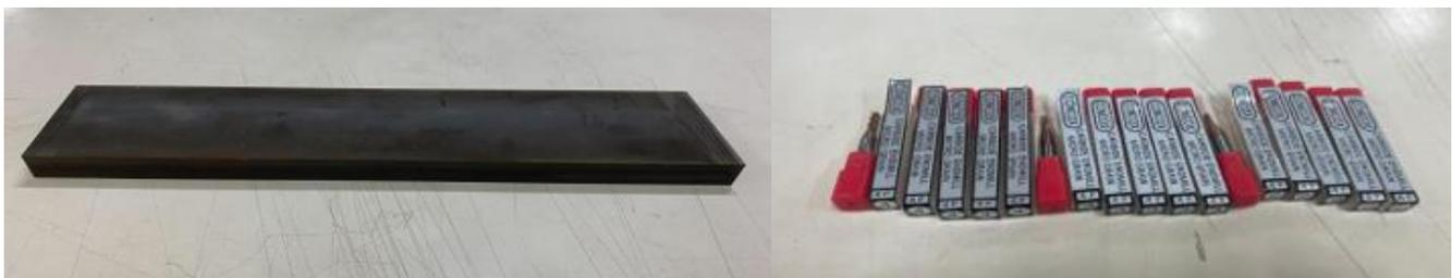
**Fig. 1.** Experimental materials and cutting tools (a) Al-nickel alloy (b) Titanium silicon tungsten steel knife.
