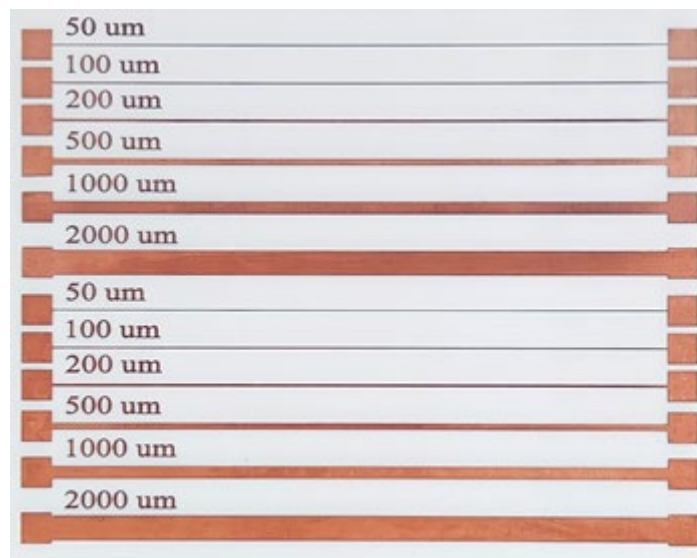
Fig. 7. Photograph of chemical copper plated contrast pattern.
