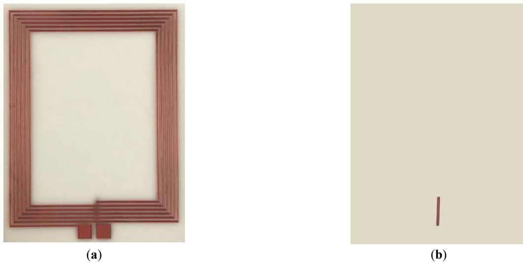
Fig. 8. Images of the NFC antenna with a line width of 400 \mu\text{m} , (a) front side, (b) back side.
