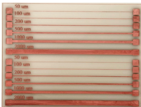
Fig. 6. Contrasted images of chemical copper plated.
