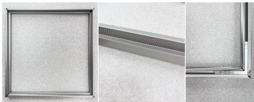
Fig. 1. Detailed waterproof design of the aluminum frame. The fine grooves and ridges on the frame enhance the waterproof effect after filling with waterproof glue.
