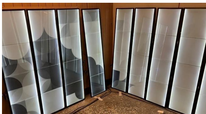
Fig. 2. E-paper aluminum frame waterproof module with LED light strips.
