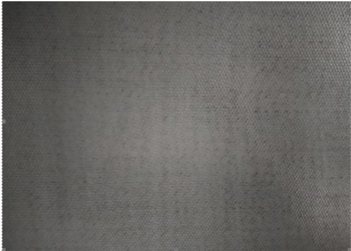
Fig. 2: Image of carbon fibre pre-impregnated fabrics fabric or pre-preg used in this study for preparation of the composite.
