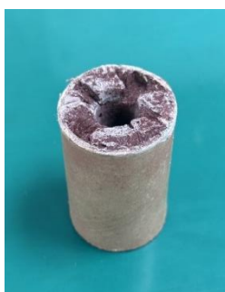
Fig. 2. KNSB solidified with drilled hole in mold.
