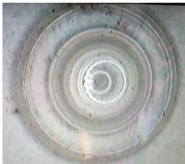
Fig. 10. Plastic lens after tuning Ultrasonic Horn.
