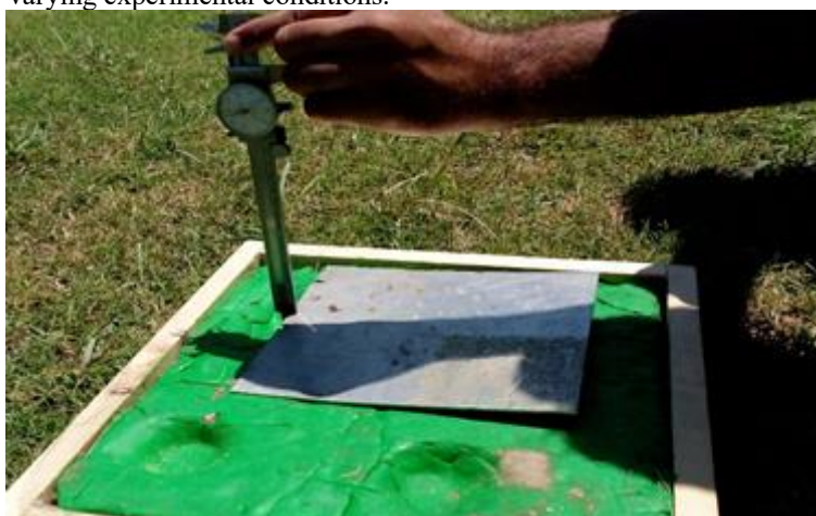
Fig. 14. BFS measurement using Roma plastilina modelling clay.
